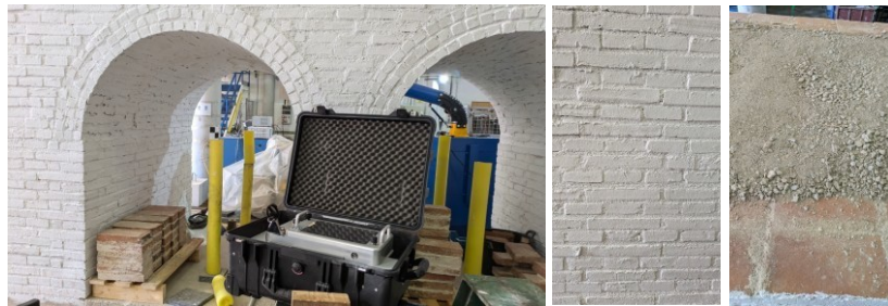
Figure 3. Experimental masonry arches and detail of the wall bricks and the sand used as filling.
