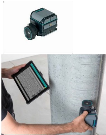
Figure 5. The GPR to be used in the project (From Screening Eagle).
