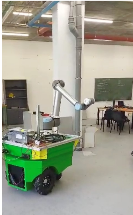
Figure 4. AgroMOBY robot with UR10 navigating in the CDEI-UPC Mobile Robotics Laboratory (MRL) space.
